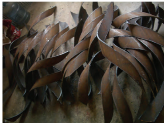
Eugene geared up his torch onto a crankshaft, rigged to turn at exactly the correct rate as the torch moved — the coils of Double Triamond , w/ Hexastix! are cut from steel pipes.
